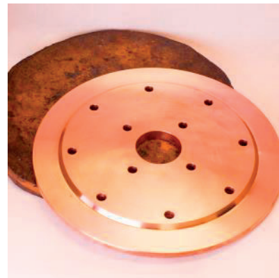
SEAM WELD WHEEL
